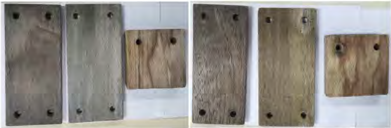
Figure 11 Surface changing after hanging test of 21 months at a sea in Qingdao
