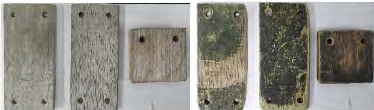
Figure 12 Surface changing after hanging test of 27 months at a sea in Qingdao
