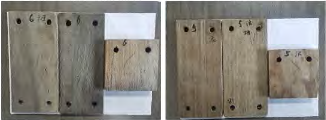
Figure 10 Surface changing after hanging test of 15 months at a sea in Qingdao
