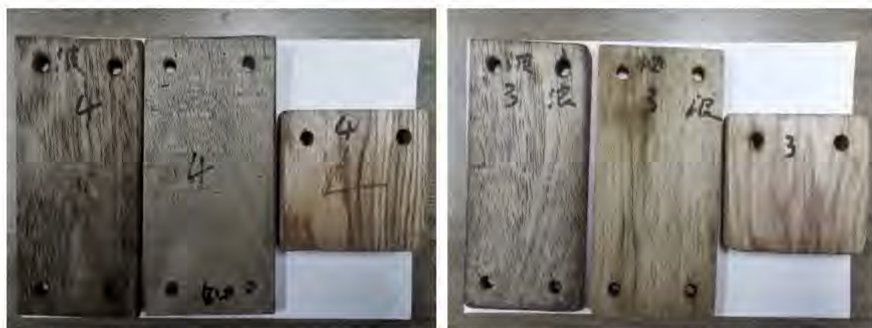
Figure 9 Surface changing after hanging test of 12 months at a sea in Qingdao
