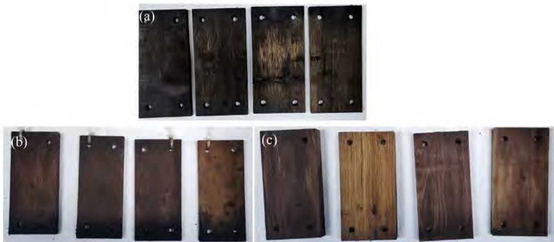
Figure 4 Salt spray test of 2560 hours
