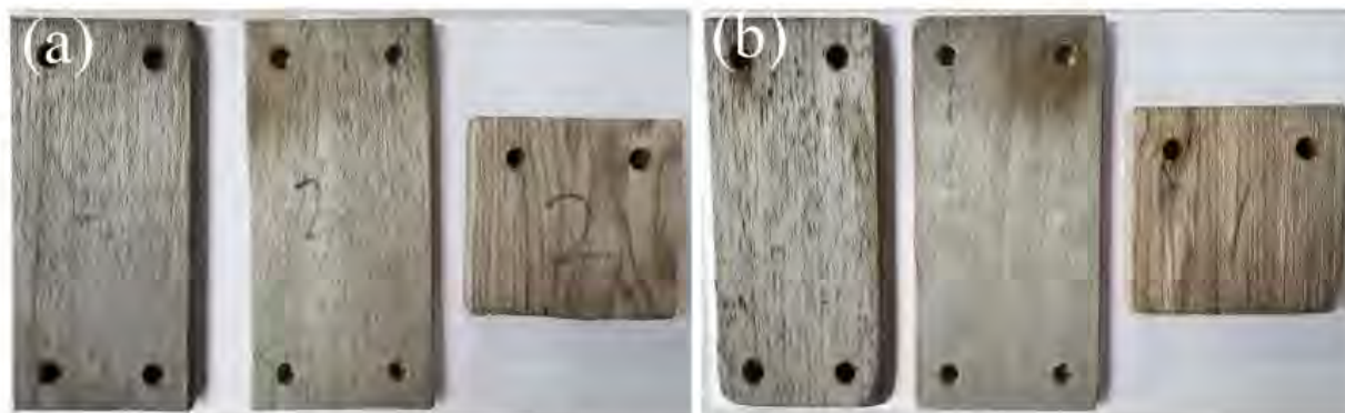
Figure 8 Surface changing after hanging test of 9 months at a sea in Qingdao
