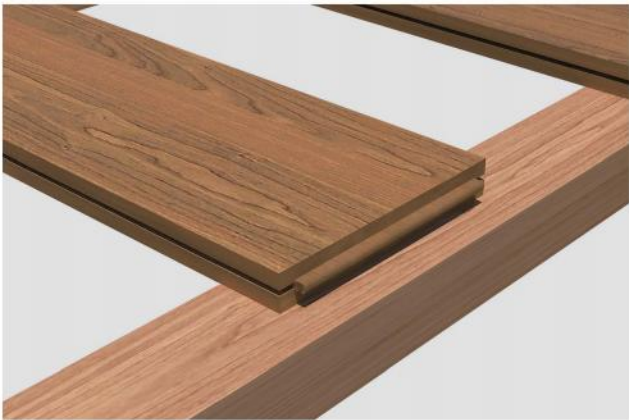
A. Starting board fixation
