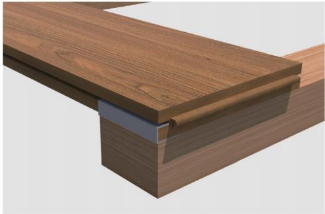
D. End on joist
