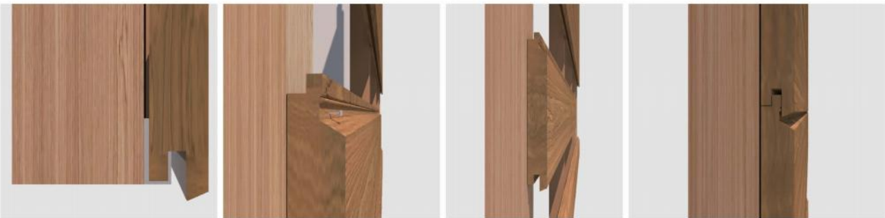
A. Starting board fixatio B. Nailing position C. Ends on joist D. Connecting method
